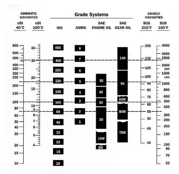
Viscosities can be related horizontally only. For example, the following oils have similar viscosities: ISO 460, AGMA 7 and SAE GEAR OIL 140.
