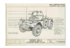
As early as 1954, a report on crew efficiency and comfort commented 'much of the vital machinery of the vehicle is housed in the crew space'. Indeed, the CES equipment list is long, but it does not include radio equipment, personal equipment for the crew or their weapons. These nine diagrams were produced early on, and thus show Larkspur radio equipment.
