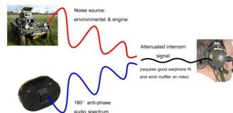
Both earshells in a headset have these small detector microphones. Both detect the noise level. Above a threshold the inbuilt frequency filter is adjusted to give the anti-phase that attenuates the noise spectrum. Each earshell will provide ANR to left & right ears, depending on the instantaneous noise on the left or right of the head.
