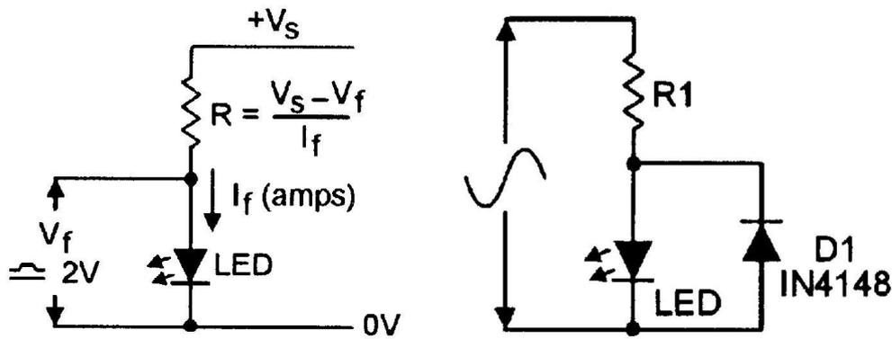
If several LEDs need to be driven from a single power source, this can be done by wiring all LEDs in series, as shown in the left-hand figure, provided that the supply voltage is significantly greater than the sum of the individual LED forward voltages. For a 24v supply, a  $V_{fn}$  value of 2v, as in the example above, the value of  $V_{ft} = 8$  volts. For a series of 20mA LEDs, the value of the resistor required is now  $800 \Omega$  rather than  $1,100 \Omega$ .
