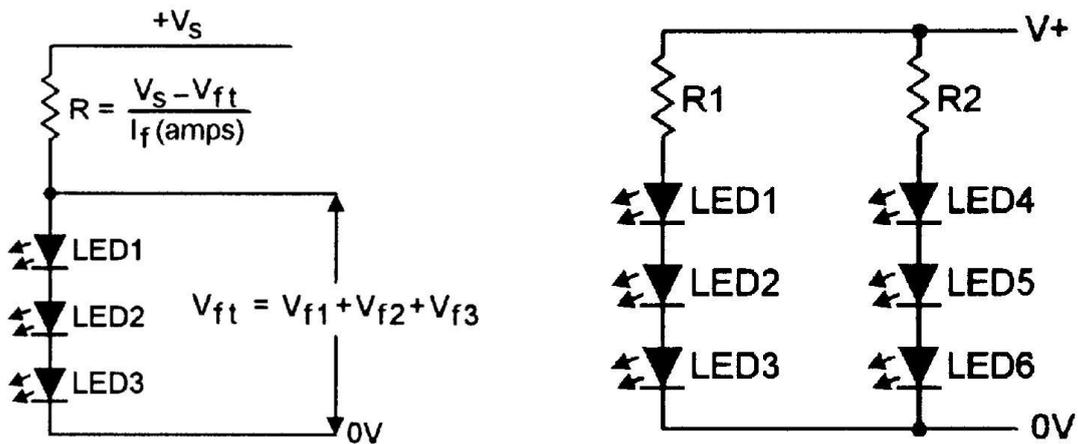
An alternative way of simultaneously powering several LEDs is to simply wire a number of the circuits above in parallel, but this is very wasteful of supply current (which equals the sum of the individual LED currents).
